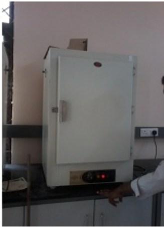
Fig-3 Oven used for heating
