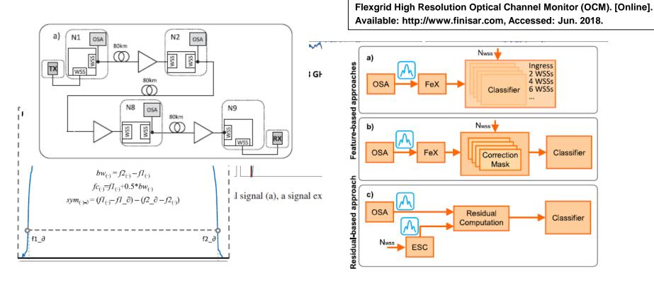
Fig. 4. Approaches to solve the filter cascading problem: (a) multi-classifier, (b) single-classifier, and (c) residual computation.
