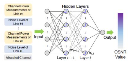
Fig. 7. Structure of the OSNR estimator.
