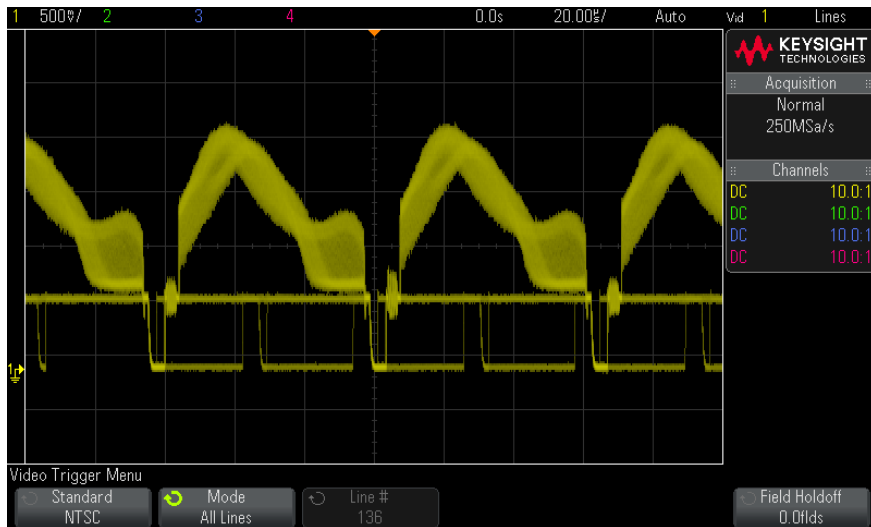
Figure 16 Triggering on All Lines
