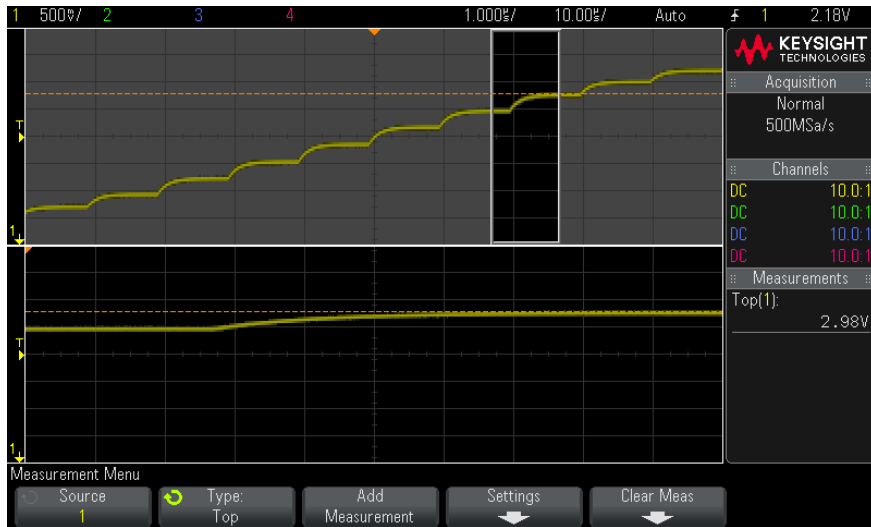
Figure 33 Isolating area for Top measurement
