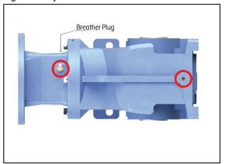
Top view, two fill / gauge / drain plug ports One with breather plug The bronze cap with rubber ring shown in Figure 3 (left) is a breather plug located in the top of the reducer as shown in this MI mounting position. If the reducer is used in another mounting position, this breather plug will need to be moved to the top fill position after the new mounting is completed. **The breather plug must always be in the top most position on the unit.**
