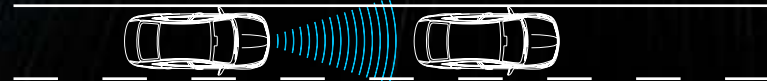
ASCC (Advanced Smart Cruise Control) A radar sensor at the front of the car monitors the gap between the vehicle ahead. The system automatically applies the brakes to maintain a pre-determined 'safe' distance and will even bring the vehicle to a complete stop, if necessary. The system will initiate take-off when car ahead moves on.
