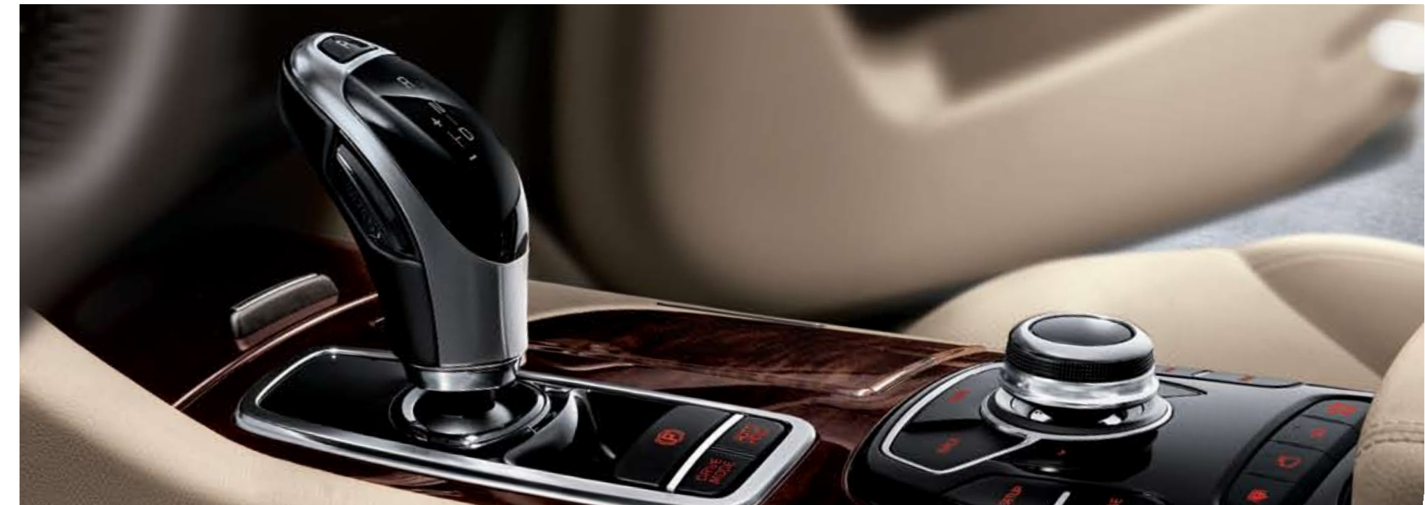
SBW (Shift-By-Wire) Electronic Gear Knob Kia Quoris features innovative SBW (shift-by-wire) technology, which removes any mechanical link between the gear selector and the gearbox. Together with a sensitive joystick control that delivers fast, smooth gear changes, SBW technology helps save space and weight while reducing engine noise in the cabin.
