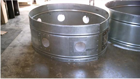
Figure 5. Lower body section with cutout holes and C-brackets installed.
