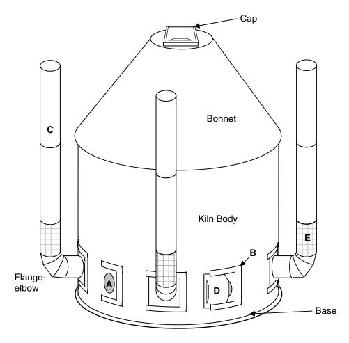
Figure 1. Modified New Hampshire charcoal kiln developed and tested at Virginia Tech.
