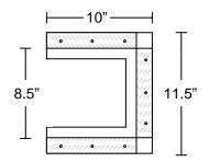
Figure 2. Detail of exhaust stack mounting bracket made from sheet metal. The side shown here faces the kiln body and is attached by nine small bolts.
