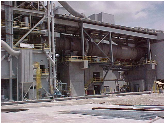
Figure 2 - 2200MTPD kiln powered by a 350hp single drive
