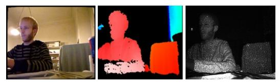
Figure 4.2: Kinect provided data: RGB image (left), depth (middle) and infrared image (right).
