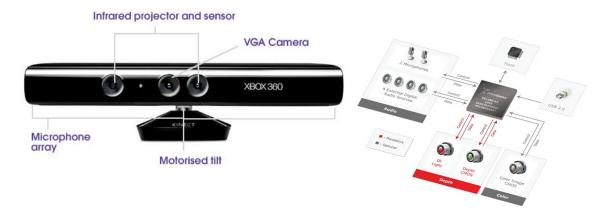
Figure 3.1: Kinect device and chip.
