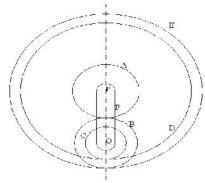
8. The sun planet gear of an epicyclic gear train, the annular D has 100 internal teeth, the sun gear A has 50 external teeth and planet gear B has 25 external teeth. The gear B meshes with gear D and gear A. The gear B is carried on arm E, which rotates about the centre of annular gear D. If the gear D is fixed and arm rotates at 20 rpm, then find the speeds of gear A and B.
