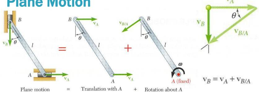
Assuming that velocity  $v_A$  of end A is known, determine velocity  $v_B$  of end B and angular velocity  $\omega$  in terms of  $v_A$ , l, and  $\theta$ .
