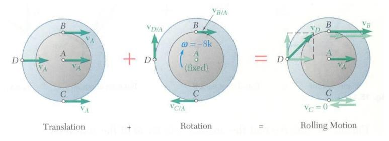
Velocity of upper rack is equal to velocity of point *B*:
