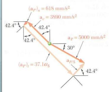
• Direction of Coriolis acceleration is obtained by rotating direction of relative velocity  $\vec{v}_{P/s}$  by 90° in the sense of  $\omega_{\rm S}$
