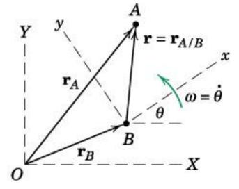
Reference Frame rotating with some accln is known as noninertial or non-Newtonian reference frame
