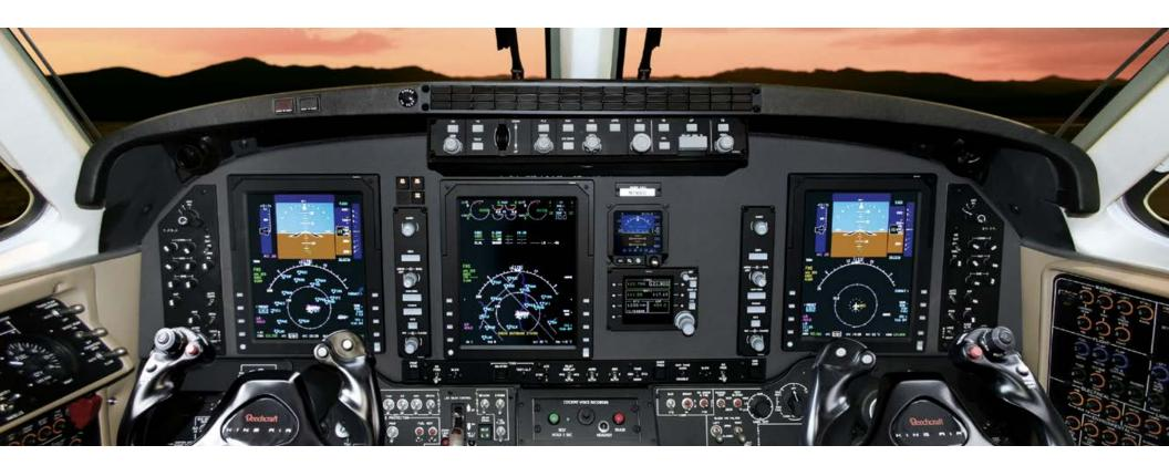
Rockwell Collins® Pro Line 21<sup>™</sup> Avionics Suite Three-Screen Electronic Flight Instrument System (EFIS) Integrated Flight Information System Engine Indicating System (EIS) Dual Air Data Computers and Altitude Encoders Dual Attitude Heading Reference Systems (AHRS) Flight Management System (FMS) with Database Input Unit MDC-3000 Maintenance Diagnostic Computer
