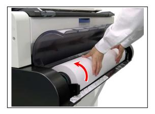
2. Rotate the roll media in the arrow direction and insert the leading edge of the roll media to the media path until it touches the feeding rollers (1).
