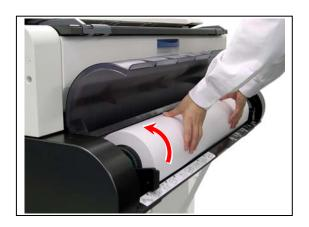
8. Rotate the roll media in the arrow direction and insert the leading edge of the roll media to the media path until it touches the feeding rollers (4).
