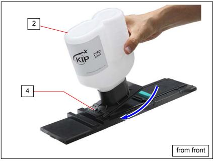
4. With pressing down the Toner Bottle (2), slide the green lever (5) to the arrow direction until it stops. When it stops, wait 10 seconds as it is.
