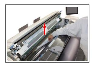
3. Put your hands on the rear rim of the scanner unit just as you hold the Upper Unit. Push the entire unit down to the arrow direction.
