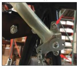
Remove air filter cover to access mounting clamp, loosen the screw far enough to remove outer wire, then remove inner wire from throttle arm. **NOTE: The end is a "Z" shape**
