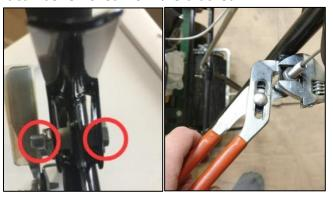
Step 4 – Remove Clutch Cable – Frame Side With the unit tipped forward and secured in place (as described on Page 1), access the connection bolt & nut and use 2 x 1/2" wrenches to loosen. NOTE: The return spring is also held in place at this connection.
