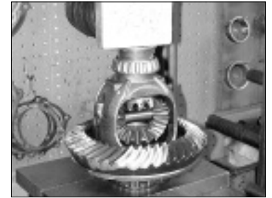
Pressing on carrier bearing
