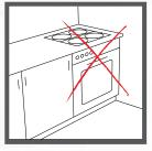
Don't place a cooktop next to a wall where it can cause overheating. Allow a minimum 450mm on either side.
