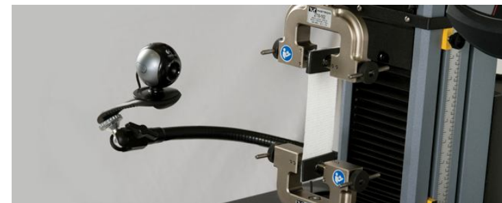
Elongation experiment of a polymeric membrane
