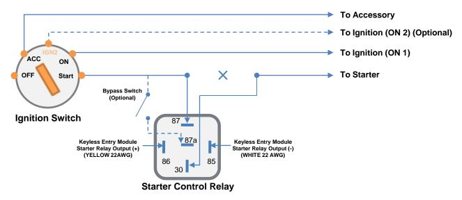
**Note:** Method 2 ignition wiring will maintain key cylinder's ACC and ON functions. However, without a valid smart access key the vehicle's starter function will be disabled by the Starter Control Relay to prevent unauthorized vehicle ignition. (This means you will not be able to start the car without the smart access key even if you use an OEM key). If desired, a switch (not included) can be added in parallel with the Starter Control Relay's normally closed pin (87a) for manual bypass.
