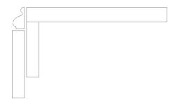
A typical baseboard configuration in our part of the country is a basic 5% x % plank with 'baseboard' molding above that. As in the case of shelf 'D' (above), these four pieces are also permanently glued together. And notice that the baseboard extends in front of the side panels. Notice also how I cut an 8" x %" notch in the back of the side panel to accommodate the baseboard.
