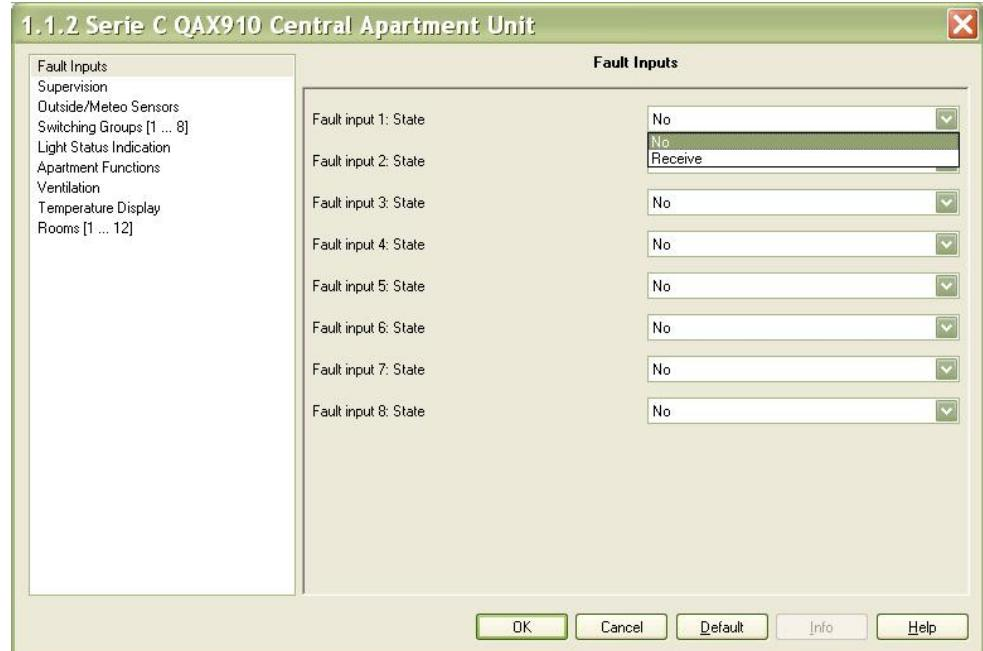
Select a parameter group in the dialog box to start parameterization. This configures or makes visible the corresponding parameters, allowing you to set the parameter values.
