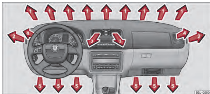
Fig. 73 Air outlet vents
