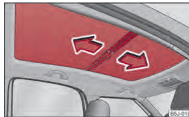
Fig. 20 Panorama roof: Open sun screen
