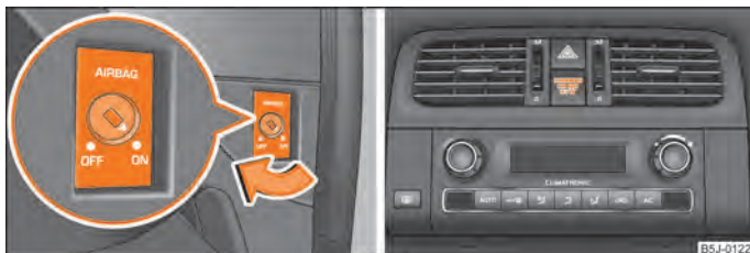
Fig. 104 Switch for the front passenger airbag/indicator light for a switched off front seat passenger airbag
