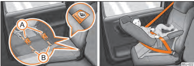
Fig. 111 Push locking eyes (ISOFIX system)/ISOFIX child seat into the installed mounting funnels
