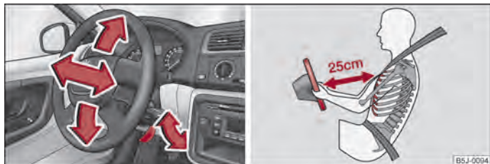
Fig. 77 Adjustable steering wheel: Lever below the steering column/Safe distance to steering wheel
