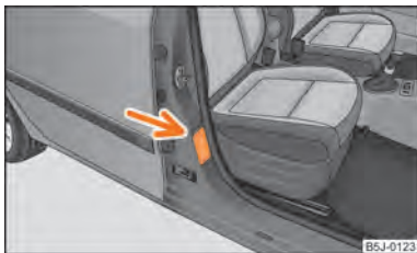
Fig. 105 Sticker on the centre column of the body on the front passenger side.
