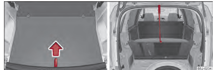
Fig. 164 Loop for raising the loading floor/Fixing the loading floor with a plastic hook
