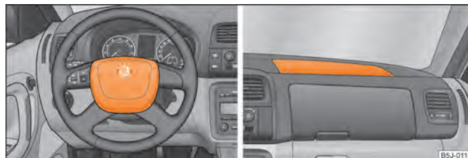
Fig. 97 Driver airbag in the steering wheel/front passenger airbag in the dash panel
