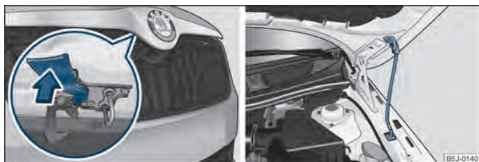
Fig. 122 Radiator grille: Locking lever/securing the bonnet with the bonnet support
