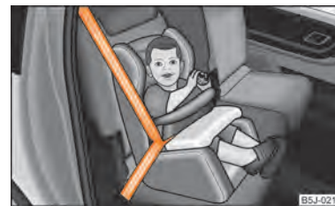
Fig. 108 Child seat with padded table in Group 1 installed on rear seat bench facing the direction of travel
