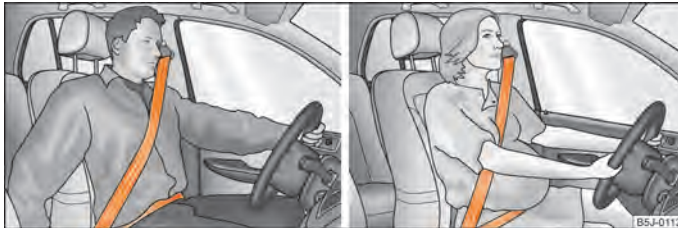
Fig. 94 Routing of belt webbing over the shoulders and the lap belt/Routing of belt webbing for an expectant mother
