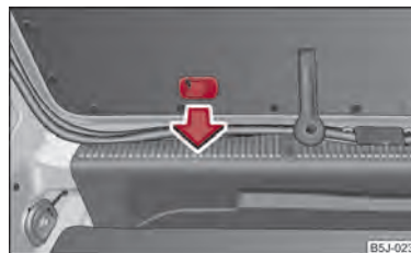
Fig. 166 Emergency unlocking of the loading area door
