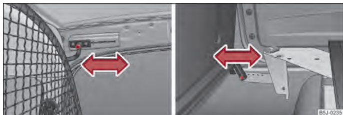
Fig. 165 Top support/bottom support of the safety partition
