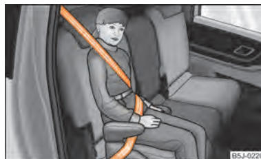
Fig. 110 Child seat in Group 3 installed on the rear seat facing the direction of travel
