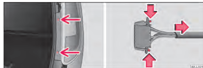
Fig. 160 Removing the rear light unit/disconnecting the plug connection
