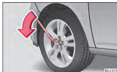
Fig. 137 : Loosening the wheel bolts ▶
