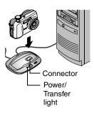
**3** Place the camera in the camera dock and push down to seat the connector.
