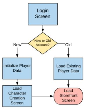
Figure 4.1: Login System flowchart
