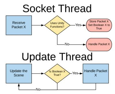
Figure 4.9: Multi-threading with Unity
