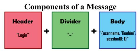
Figure 4.10: The construction of a Login Message
