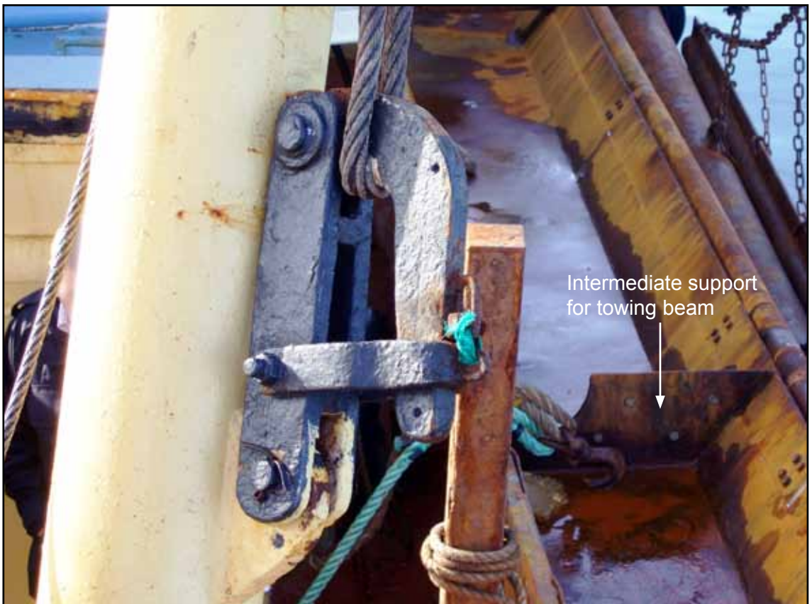
Intermediate supports for towing beam cradle arrangement
