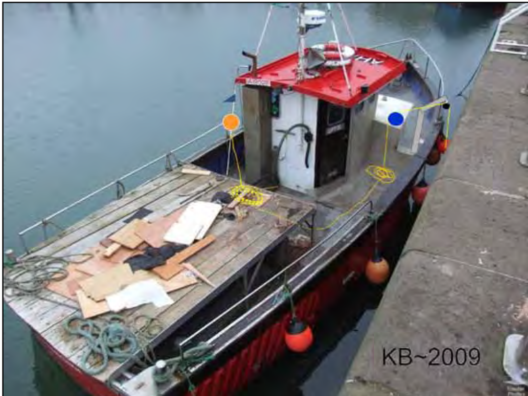
Representation of dhan buoy in recovered position with section of rope obscured between shooting table and wheelhouse
