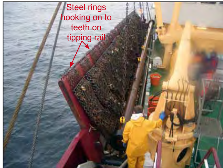
Tipping rail mechanism
