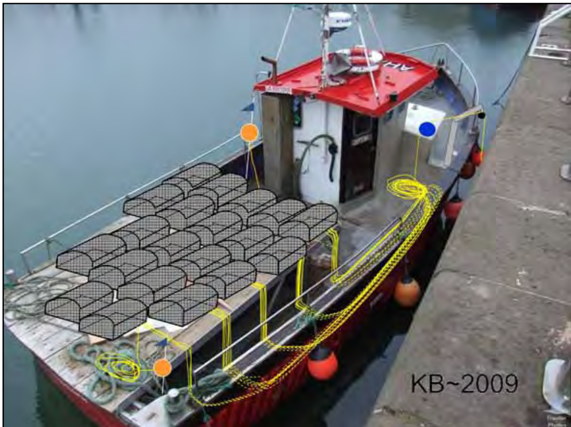
Representation of fleet of recovered creels stowed on the shooting table in preparation for shooting
