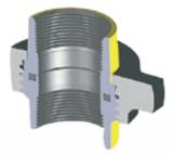
**KPL'S** Figure 300 is manufactured from carbon steel. This Flat-Face type union has an O-Ring seal. Recommended for use where straight breakout of pipe segments is required. Suitable for water, oil, or gas service at pressures up to 12,500 PSI NSCWP. Please note that colors vary per pressure rating.
