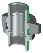
**KPL'S** Figure 1003 (Mis-aligning Union) has NPT or Butt Weld Ends. It is constructed of Forged Alloy Steel, and comes with a Buna N O-Ring. Recommended for high pressure water, oil, mud or gas service where alignment of piping is a problem, with up to 7 1/2° angular adjustment from center (15° total).
