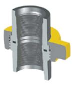
**KPL'S** Figure 201 has EUE 8 Round Tubing Threads. This union is a Flat-Face type union that utilizes an O-Ring seal. The Figure 201 is available in 2 3/8" EUE and 2 7/8" EUE. Like parts in each size are interchangeable with other manufacturers' unions. Recommended for water, oil or gas service to 3,000 PSI NSCWP.
