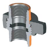
**KPL'S** Figure 602 has a replaceable lip-type seal ring of Buna-N specifically designed to minimize fluid flow turbulence. The replaceable lip-type ring also provides a pressure seal and protection for the metal-to-metal seating surfaces. These unions are recommended for manifold and truck mounting where size and weight are critical. Recommended for air, water, oil, gas or mud service up to 6,000 PSI NSCWP.
