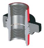
**KPL'S** Figure 400 features a precision ball and cone sealing surface for sure metalto-metal seal. Recommended for water, oil and gas service to 4,000 PSI NSCWP.
