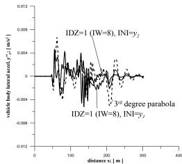
Fig. 14: Results of simulation for vehicle body (lateral acceleration) for the optimised TCs and 3<sup>rd</sup> degree parabola: 10<sup>th</sup> (<u>Routes 5</u> and <u>6</u>)
