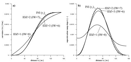
Fig. 11: <u>Route 6</u> - features of TCs: a) curvatures of the initial and optimised TCs, b) superelevation ramps' slopes
