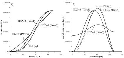
Fig. 5: <u>Route 3</u> - features of TCs: a) curvatures of the initial and optimised TCs, b) superelevation ramps' slopes
