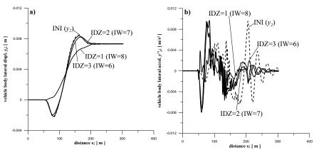
Fig. 12: <u>Route 6</u> - results of simulation for vehicle body for the initial and optimised TCs: a) lateral displacement, b) lateral acceleration
