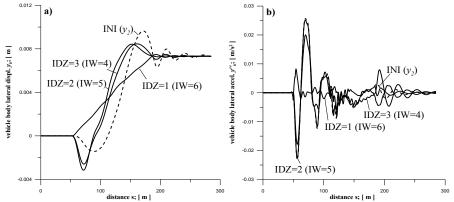
Fig. 8: <u>Route 4</u> - results of simulation for vehicle body for the initial and optimised TCs: a) lateral displacement, b) lateral acceleration
