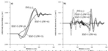
Fig. 6: <u>Route 3</u> - results of simulation for vehicle body for the initial and optimised TCs: a) lateral displacement, b) lateral acceleration
