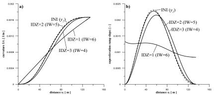
Fig. 7: <u>Route 4</u> - features of TCs: a) curvatures of the initial and optimised TCs, b) superelevation ramps' slopes
