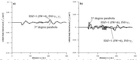
Fig. 13: Results of simulation for vehicle body (lateral acceleration) for the optimised TCs and 3<sup>rd</sup> degree parabola: a) 6<sup>th</sup> (Routes 1 and 2), b) 8<sup>th</sup> (Routes 3 and 4)
