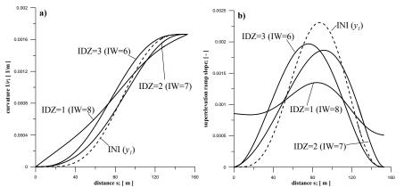
Fig. 9: <u>Route 5</u> - features of TCs: a) curvatures of the initial and optimised TCs, b) superelevation ramps' slopes
