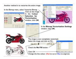
Export the image as a DXF file to the laser cutter. Place the material into the laser and follow the settings and safety rules in the handbook to cut it out correctly.
