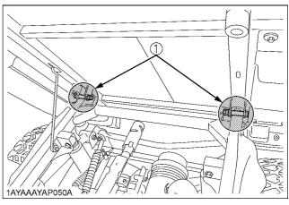
(1) Cargo bed pivot (spray type grease)
