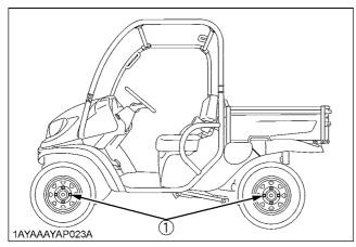
(1) Torque wheel bolts to 108.4 to 121.9 N-m (11 to 12.4 kgf-m) (80 to 90 ft-lbs.)
