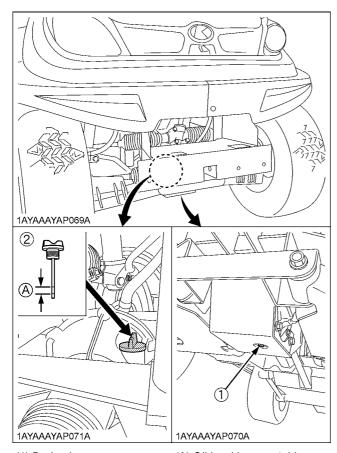
(1) Drain plug(2) Filling plug with dipstick
