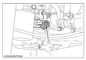
(1) Bypass link (spray type grease)
