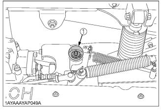
(1) VHT link (Grease fitting)
