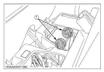
(1) Battery terminals (spray type grease)
