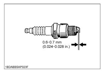
8. Reinstall the spark plug into the cylinder head.
