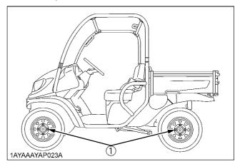
(1) Torque wheel bolts to 108.4 to 121.9 N-m (11 to 12.4 kgf-m) (80 to 90 ft-lbs.)
