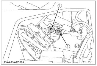
(1) Parking brake pivot (spray type grease)
