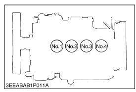
The cylinder numbers of kubota diesel engine are designated as shown in the figure.
