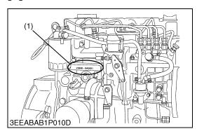
When contacting the manufacture, always specify your engine model name and serial number.
