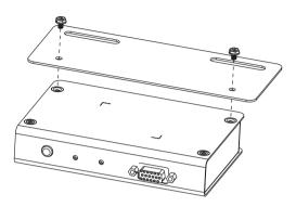
3. Screw the bracket into any convenient location on the rack.
