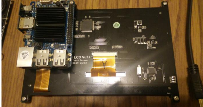
Figure 2 - Attaching the ODR0ID-C1+ on the back of the Vu7 Plus
