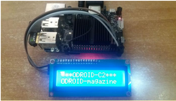
Figure 4 - LCD screen displaying a dual-line message
