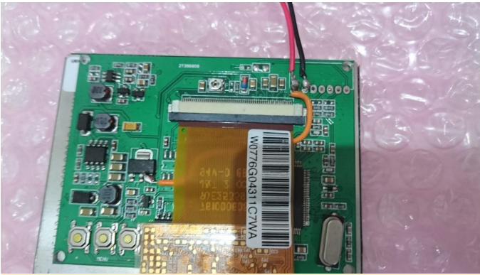
Figure 6 - Closeup of the ODR0ID 5V wiring
