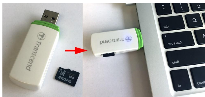
Figure 3 - Inserting the USB adapter and microSD card in the computer
