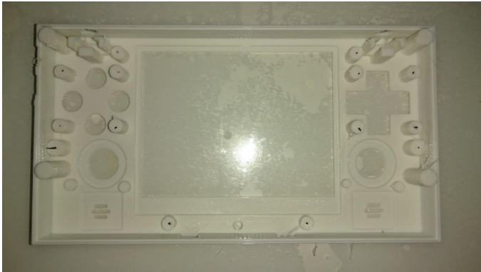
Figures 2 and 3 - Back internal view of the case. You can see batteries space at the bottom and some striations for CPU + GPU thermal dissipation.
