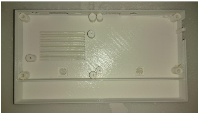
Figures 2 and 3 - Back internal view of the case. You can see batteries space at the bottom and some striations for CPU + GPU thermal dissipation.
