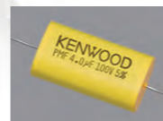
Hi-Grade Film Condenser improves higher frequency performance.
