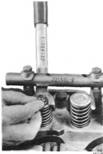
FIGURE 13 — Valve Spring Removal
