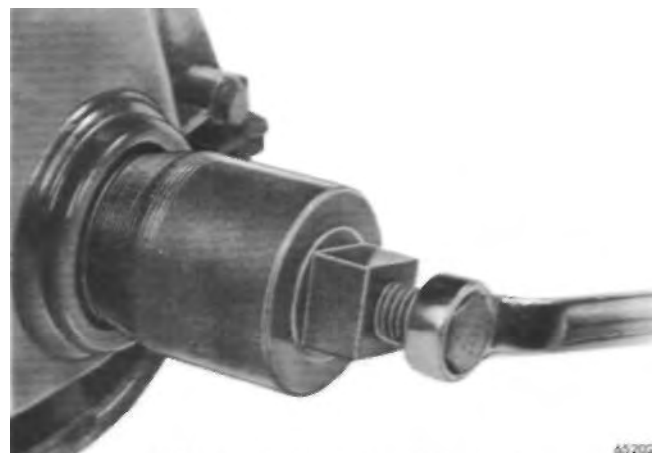
FIGURE 31 — Removing Timing Chain Cover Oil Seal with J-9256 Remover
