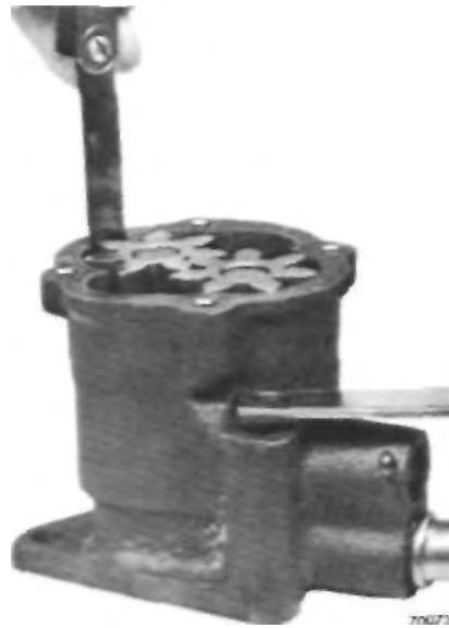
FIGURE 36 — Measuring Oil Pump Gear to Body Clearance
