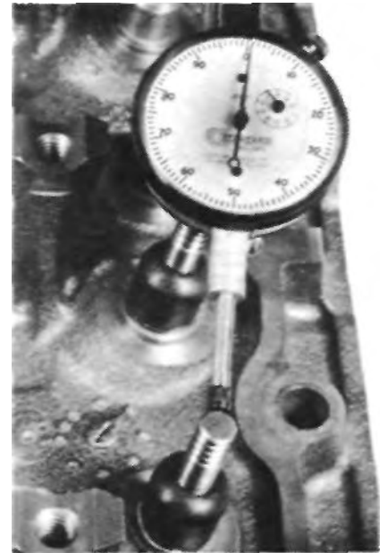
FIGURE 19 — Checking Valve Guide Clearance
