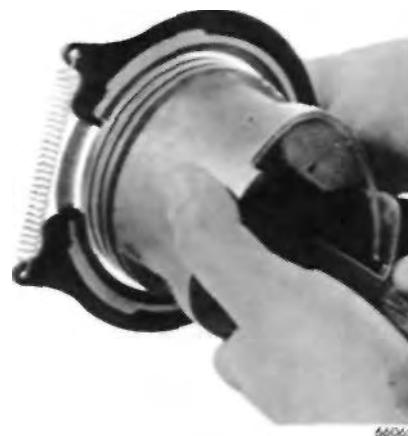
FIGURE 46 — Installing Compression Rings on Piston Using Tool J-8028
