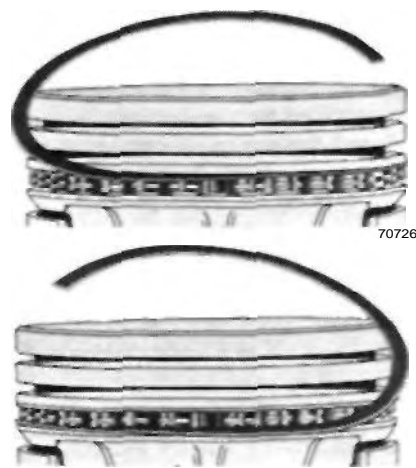
FIGURE 44 - Oil Control Ring Installation
