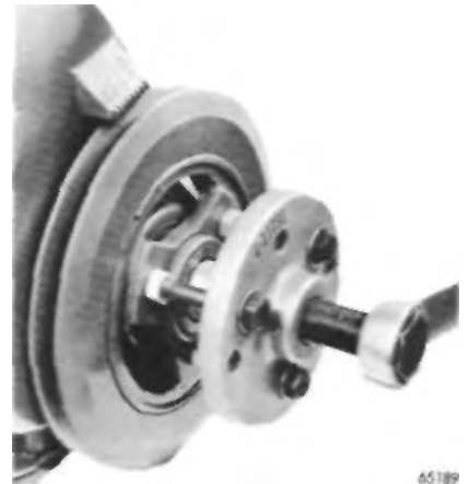
FIGURE 26 — Removing Vibration Damper Assembly with Tool J-21791
