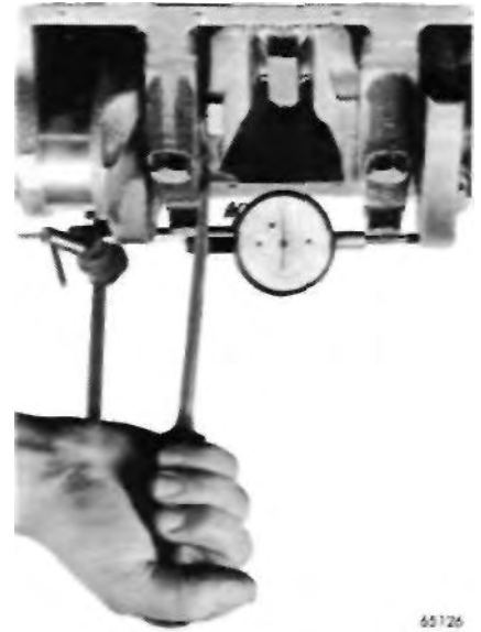
FIGURE 50 - Checking Crankshaft End Play
