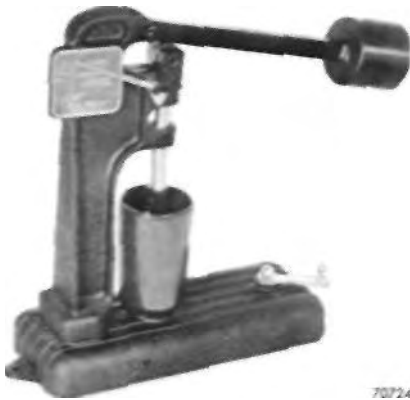
FIGURE 24 - Testing Valve Tappet "Leak-Down" with J-5790
