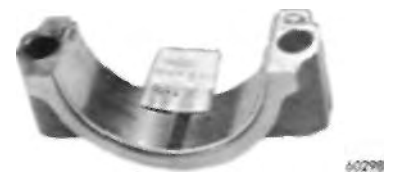
FIGURE 39—Checking Bearing Clearance with Plastigage
