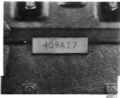
FIGURE 1 - Engine Code Typical Location
