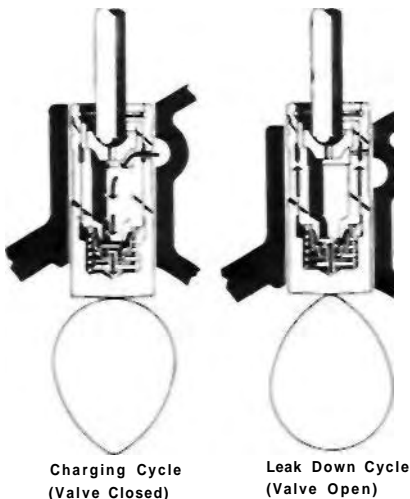
FIGURE 21 - Hydraulic Tappet Operation Cycle
