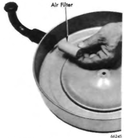
FIGURE 8 — Removing Air Inlet Filter
