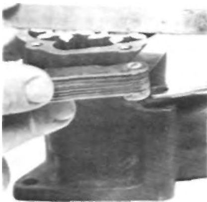
FIGURE 35 — Measuring Oil Pump Gear End Clearance
