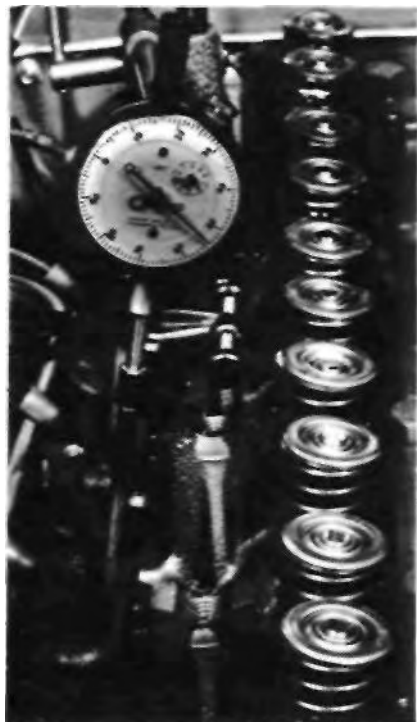
FIGURE 34 - Installation of Dial Indicator for Checking Cam Lobe Lift
