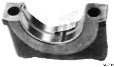
FIGURE 49 - Checking Main Bearing Clearance With Plastigage
