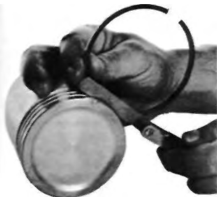
FIGURE 42 - Checking Ring Side Clearance
