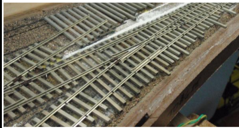
Tom Piccirillo uses wooden ties and code 100 rail for his "O" Scale Somerset County Traction System and hand spikes each tie. ►
