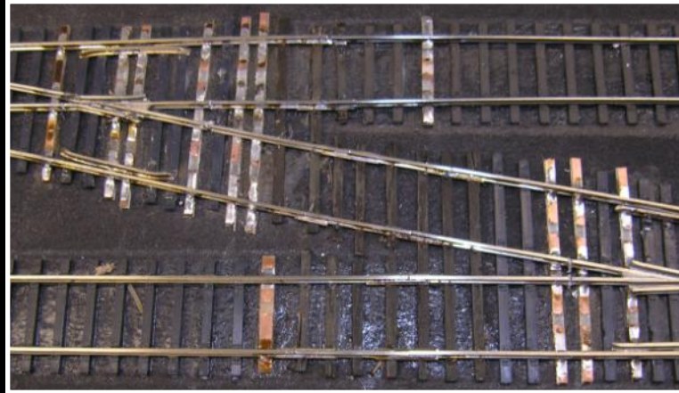
Tony Koester uses Central Valley turnout strips with Clover house throw bars and Details West cast frogs and then hand spiked on his NKP railroad Sub Division. ►
