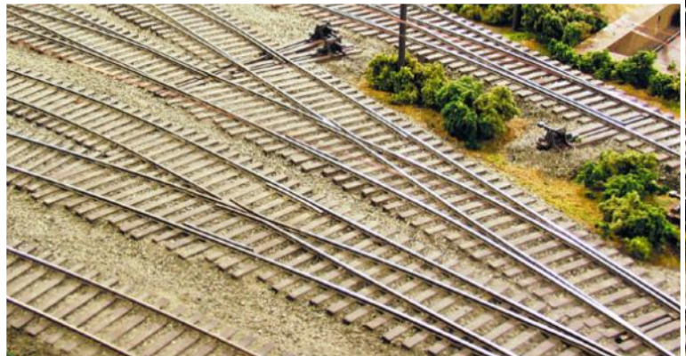
◀ Tom Wortmann uses Central Valley tie strips and BK Industries switch kits modified with PC ties from Clover house. Code 70 rail is then spiked and soldered on the MS&K railroad.
