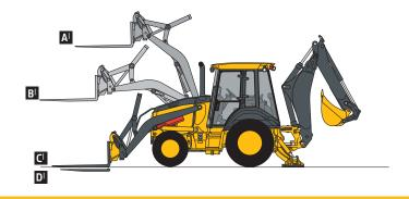
Lift capacities are over-end values in kg (lb.) according to SAE J31. Figures listed are 87% of the maximum lift force available. Calculated with 610-mm x 0.21-m<sup>3</sup> (24 in. x 7.5 cu. ft.) bucket. Bucket impacts overall lift capacity. STANDARD LIFT STANDARD LIFT
