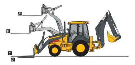
Lift capacities are over-end values in kg (lb.) according to SAE J31. Figures listed are 87% of the maximum lift force available. Calculated with 610-mm x 0.21-m<sup>3</sup> (24 in. x 7.5 cu. ft.) bucket. Bucket impacts overall lift capacity. STANDARD LIFT
