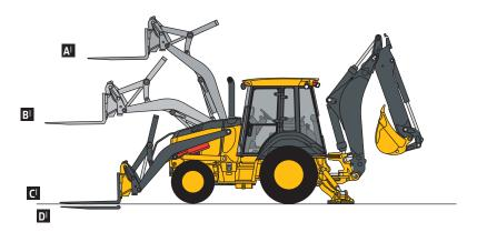
Lift capacities are over-end values in kg (lb.) according to SAE J31. Figures listed are 87% of the maximum lift force available. Calculated with 610-mm x 0.21-m<sup>3</sup>
