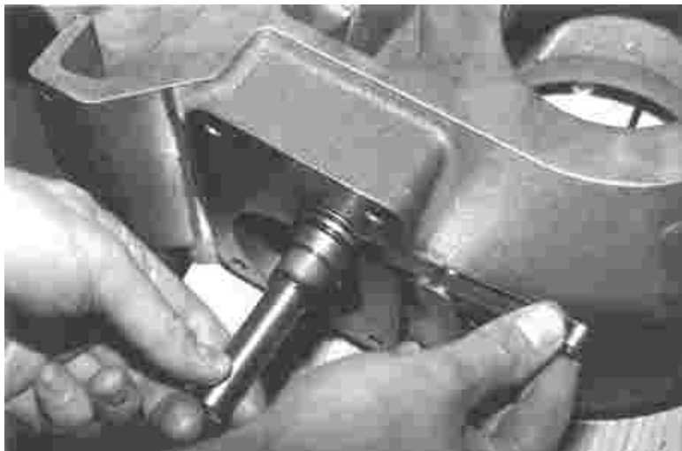
Figure 26 - Using feeler gauge to measure gap between actuator Housing face and Handwheel Bushing
