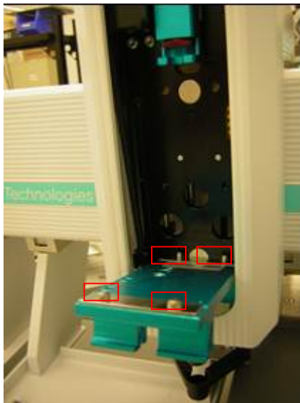
Figure 5 – Left: four pins align the syringe holder. Figure 6 – Right: ensure that holder is the right way up.
