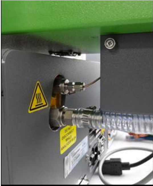
Figure 44.1 - Left, 1/16 th inch tube connection to analyzer.
