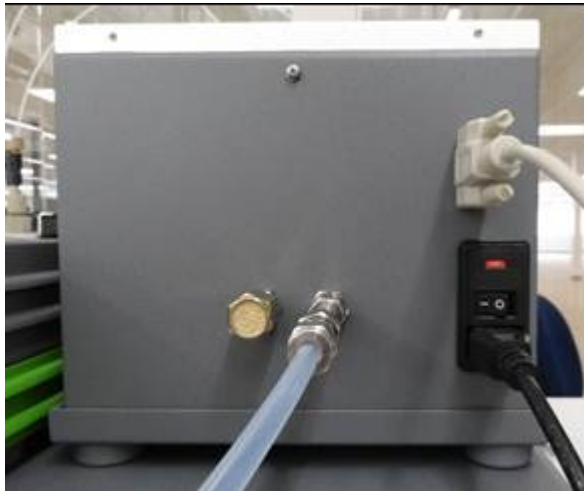
Figure 33 - Back of the SDM. Black Cord connects to Power. The Grey serial cable connects to the COM 1 Port of the Analyzer. The Semi transparent gas tube connects to the Drierite.
