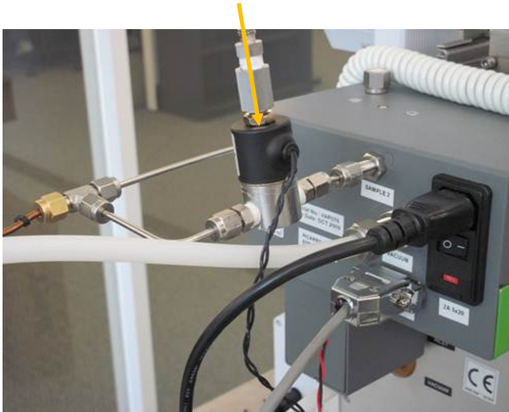
Figure 27 – Vaporizer Switching Valve Connected to the Vaporizer. The orange arrow signifies the direction of ambient vapour source.
