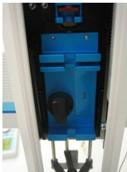
Figure 6.1 – Left: four pins align the syringe holder. Figure 6.2 – Right: ensure that holder is the right way up.
