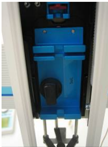
Figure 5 – Left: four pins align the syringe holder. Figure 6 – Right: ensure that holder is the right way up.
