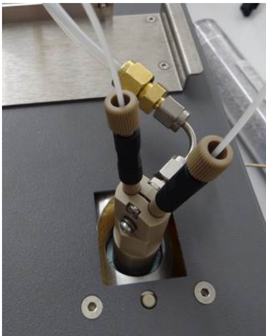
Figure Above: SDM Injector Head Assembly after being connected to the Vaporizer.
