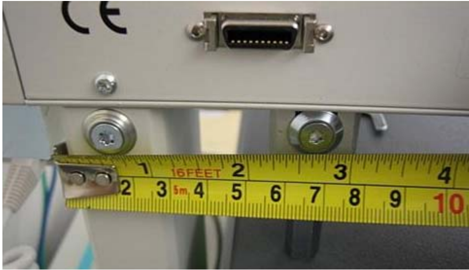
Figure 11 - The correct positioning for the vaporizer holder relative to the Autosampler.
