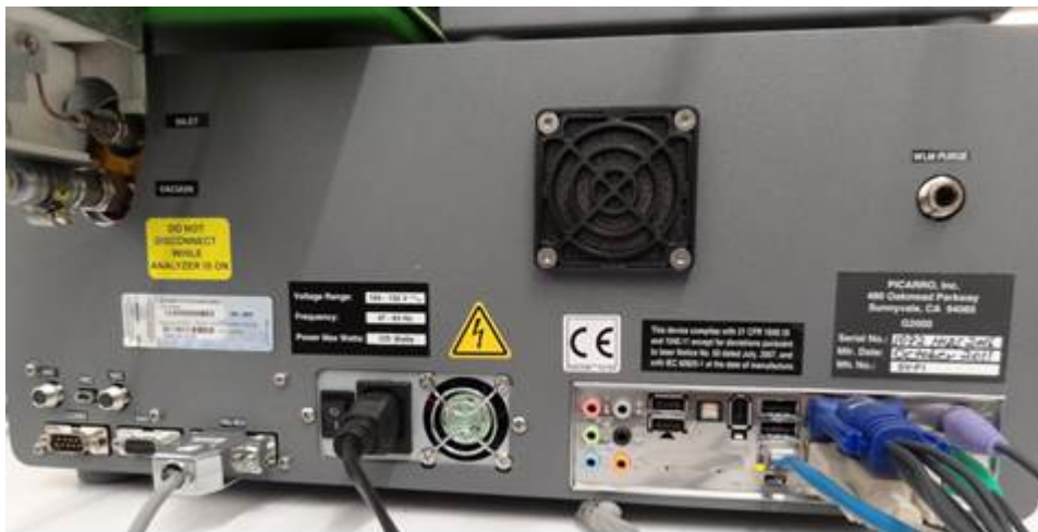
Figure 34: Back of the Analyzer. Com1 Port is underneath the port where the blue/black cable(the other end of the cable is connected to the monitor) is connected to in the image above.
