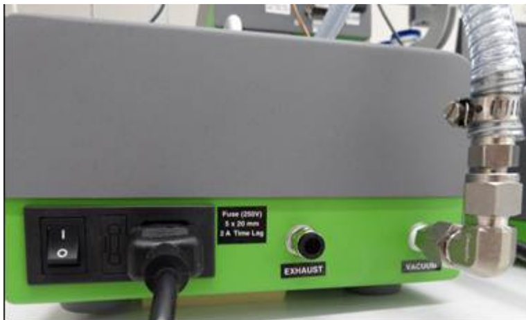
Figure 1.2 - Back of the External Vacuum Pump showing electrical and gas connections.
