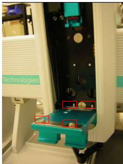
Figure 6.1 – Left: four pins align the syringe holder. Figure 6.2 – Right: ensure that holder is the right way up.
