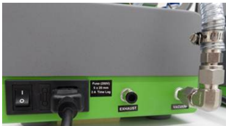
Figure 30 - Back of the External Vacuum Pump showing electrical and gas Connections.
