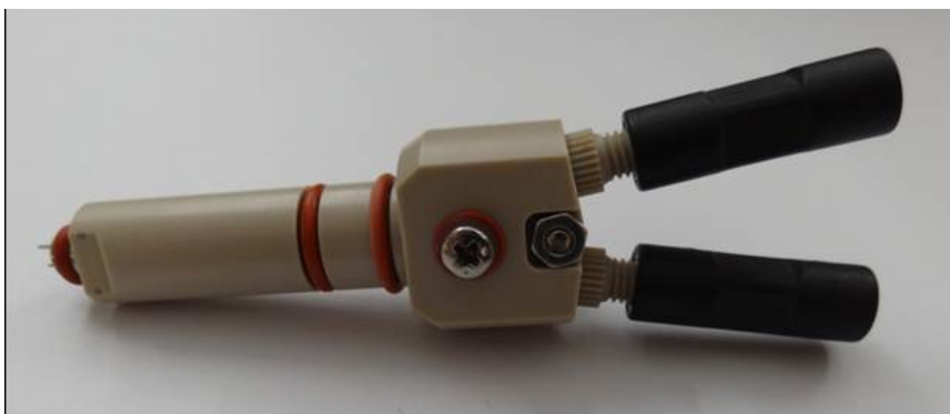
Figure 41.2: What you should see after the completion of Step 2: Slide two needles into each holes on the body of the Injector Head Assembly.
