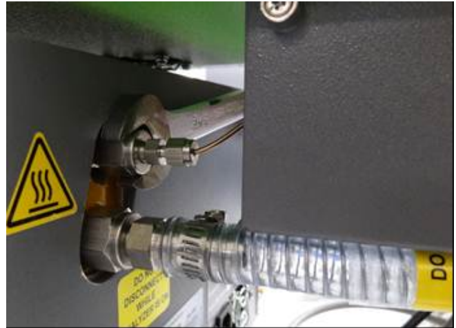
Figure 44.1 - Left, 1/16 th inch tube connection to analyzer.
