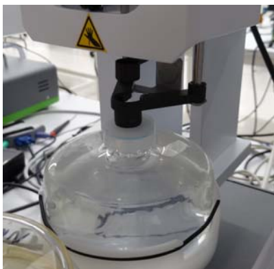
Figure Above: Bottom of assembly aligned with the wash station.
