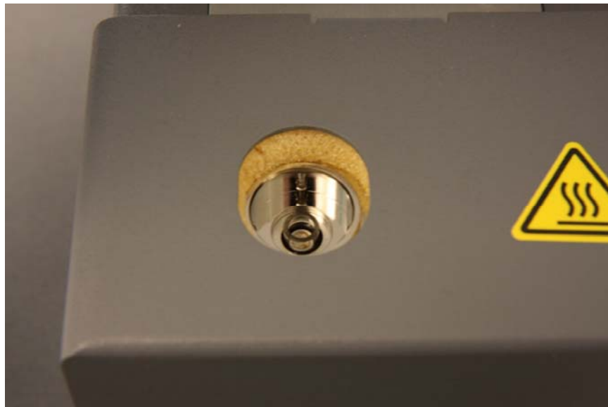
Figure 18. Close-up of vaporizer liner inside vaporizer.
