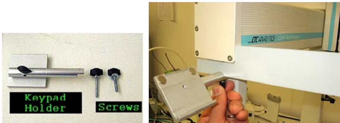
Figures 22 - Keypad holder, protective guard fittings and orientation
