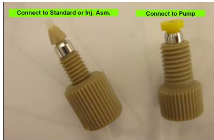
Figure 39: Two different ends of a liquid tubing. The one on the left attaches to the liquid bag or the Injector Head Assembly. The one on right attaches to the ceramic pumps.
