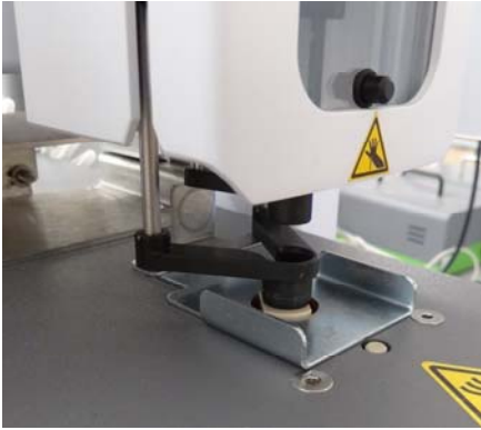
Figure Above: Bottom of assembly aligned with the injector port of vaporizer
