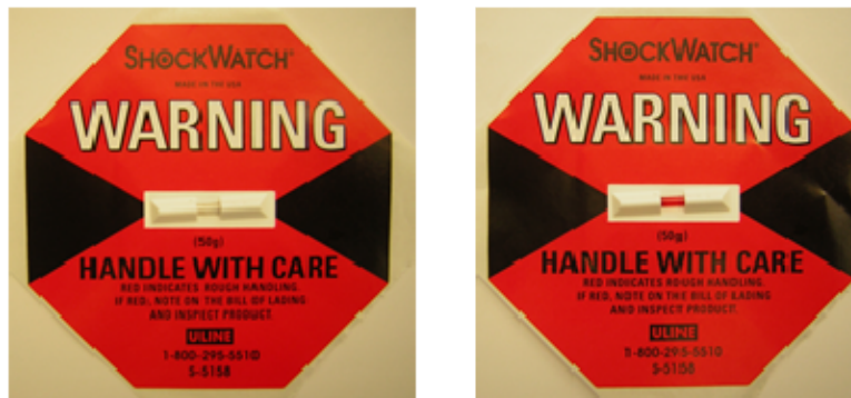
Figure 1, 2. Outer ShockWatch®. Left, untripped, right, tripped.
