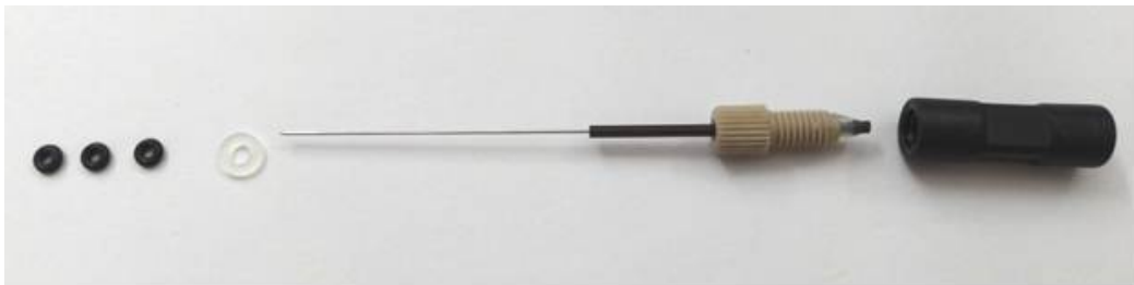
Figure 41.1: From left to right: 3 Orings, 1 spacer, 1 needle, and 1 needle union. Screw on the union on the right side of the needle as shown above. Slide in the spacer and three O-rings on the left side of the needle as shown above. Make two needle assemblies. (Step 1)
