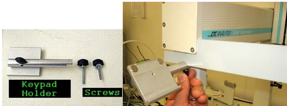
Figure 8.1, 8.2 - Keypad holder, protective guard fittings and orientation
