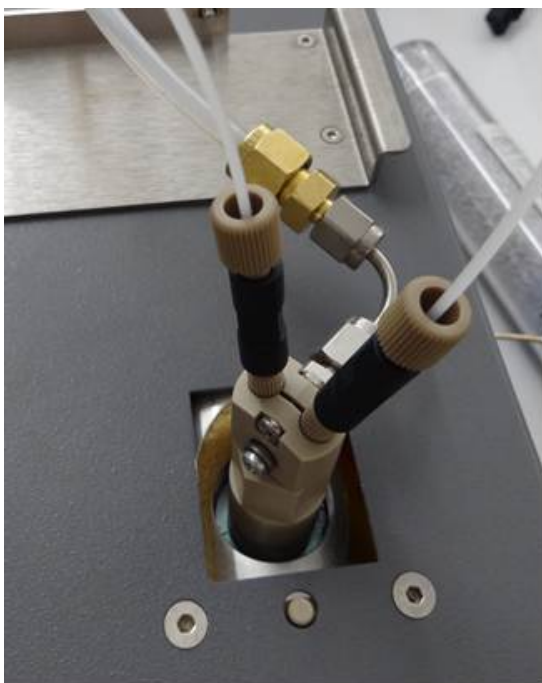
Figure 41.5: SDM Injector Head Assembly after being connected to the Vaporizer. Notice how the elbow tube and the adaptor is attached to the gas inlet of the injector port assembly (Step 4, Step 5).
