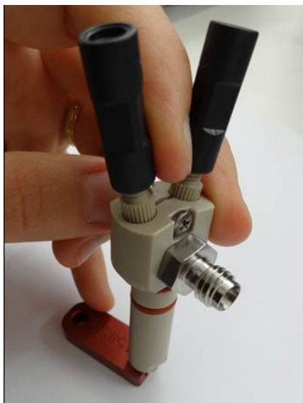
Figure 41.3: How to adjust the depth of the two needles at the bottom of the injector port assembly using a spacer tool (Step 3).
