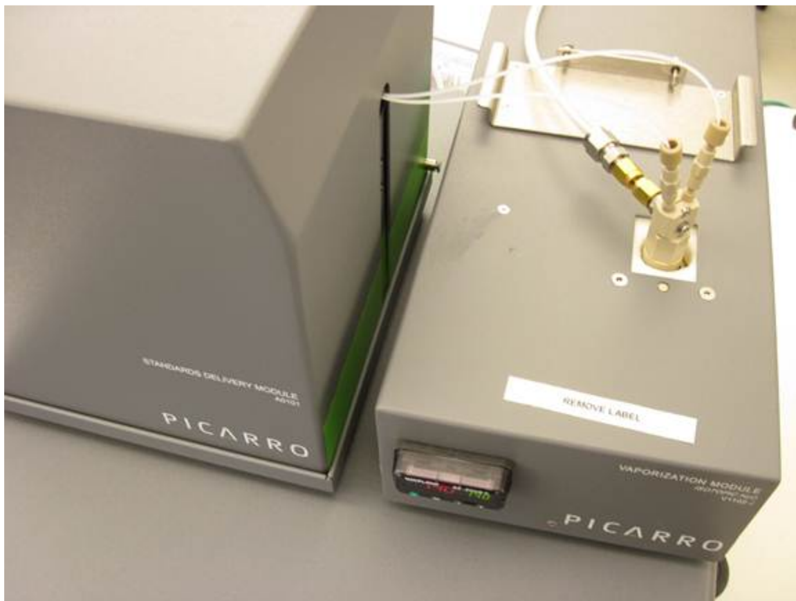
Figure 45 – After the Injector Head Assembly has been inserted into the Vaporizer. To the left is the SDM. To the right is the Vaporizer. At the bottom of the Vaporizer and the SDM is the Analyzer.
