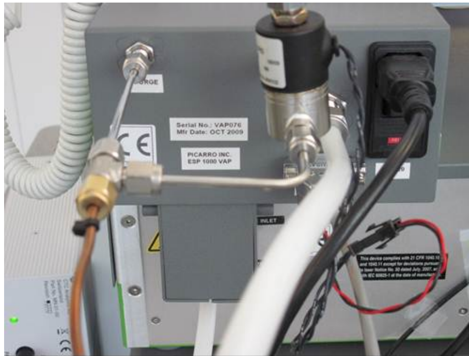
Figure 29: Pictures showing the connections on the back of the vaporizer:
