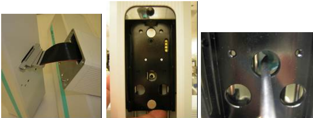
Figures 3, 4, 5 - From left to right: Connect the ribbon cable and align the two pins. Lift the black plate and look through the top central hole to align the threaded hole. Use the Torx driver to push the screw through and tighten.
