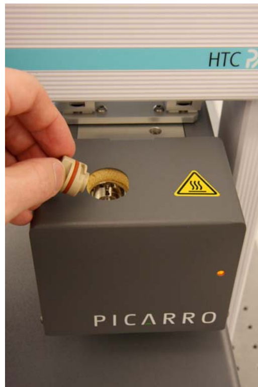
Figure 16. Vaporizer with needle guide removed. Needle guide should be turned ¼" turn counter clockwise to release.
