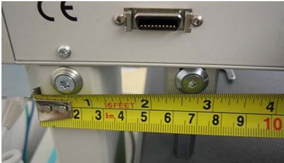
Figure 11.2 - The correct positioning for the vaporizer holder relative to the Autosampler.
