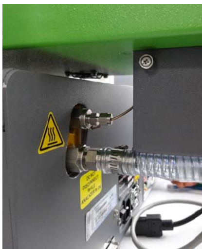
Figure 15.1 –Left , 1/16 th inch tube connection to analyzer. Figure 15.2 - Right, Hand Screw and then tighten with a wrench.
