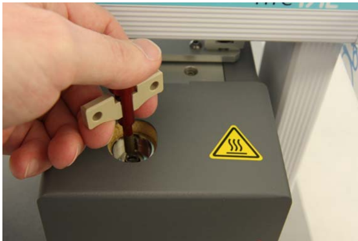
Figure 17. Vaporizer liner extraction tool being used to remove glass vaporizer liner.
