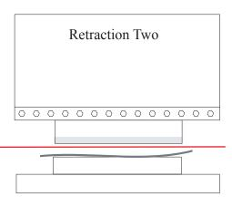
Retracts until the beam is not broken by the material.
