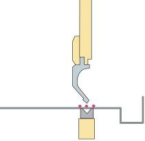
Laser beam detects part and allows the machine to continue forming.
