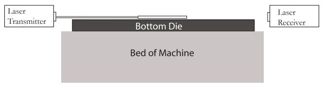
Part detection: Part blocks enough of the beam to prevent the laser beam from reaching the receiver, in this condition the "Part has been detected", no error. If the part is not detected you will receive an error "PART NOT DETECTED" and the ram will stop and or return to its' up position.
