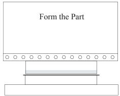
Press the foot switch a 4th time and the ram will descend in slow speed, the laser beam will be ignored and the part can be formed without interference.
