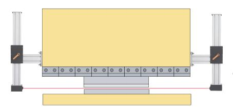
When the ram is descending, the machine is guarded by the *Laser Sentry*. At 1/2 inch or greater above the part being formed, the *Laser Sentry* shifts the machine's ram into slow speed. (down acting machines).
