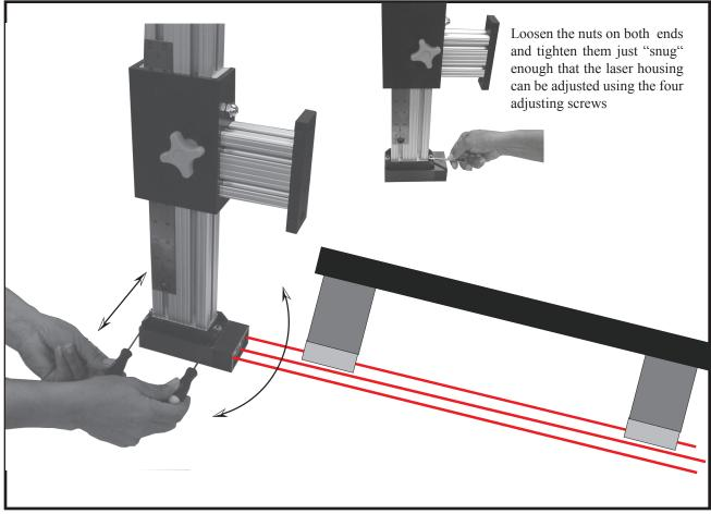
By loosening the nuts slightly you can micro-adjust the skew of the beams. Using two allen wrenches loosen the micro adjusting screws in the direction you want to move the head and tighten the opposite screws until reaching correct alignment. Tighten the opposing screw and recheck alignment. Micro-adjust the screws until you have perfect alignment and both screws are "snug" tight.
