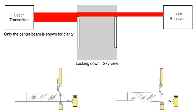
In Box Mode the front laser beam is muted. As long as the box flange is held against the back stop and the vertical flange is only partially blocking the center beam the box or tray can be formed.
