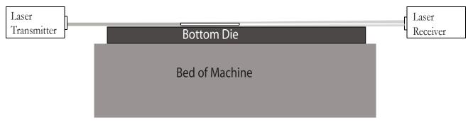
If you are forming small thin parts, always teach the Laser Sentry the part surface with the part in the same place where you are going to form the part.
