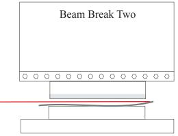
Laser beam encounters wavy material the second time.
