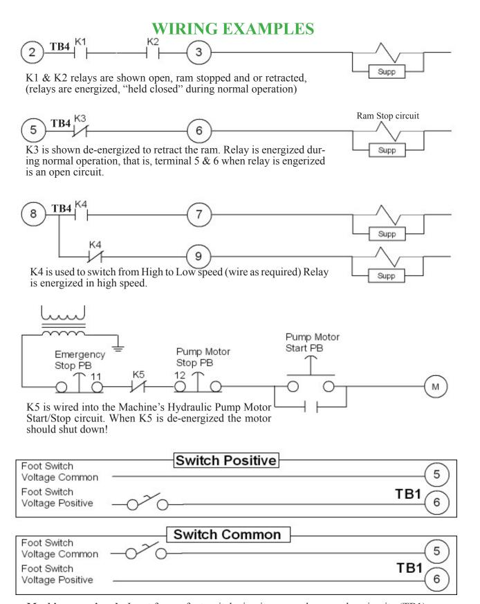
Machine run signal - Input from a foot switch circuit or ram closure valve circuit. (TB1) Terminal #5 & 6: The Board is supplied with a AC input module installed (Yellow). This module uses 90 to 140VAC. Connect the Common to TB1 (5). Connect the Positive from the N/O circuit to TB1 (6). If you require a DC input, install the (White) DC module. Wiring is the same except it requires 3 to 32VDC.
