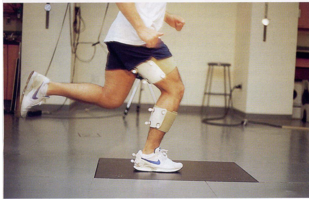
The runner traverses a 75 ft. runway contacting the force plate at its centre.
