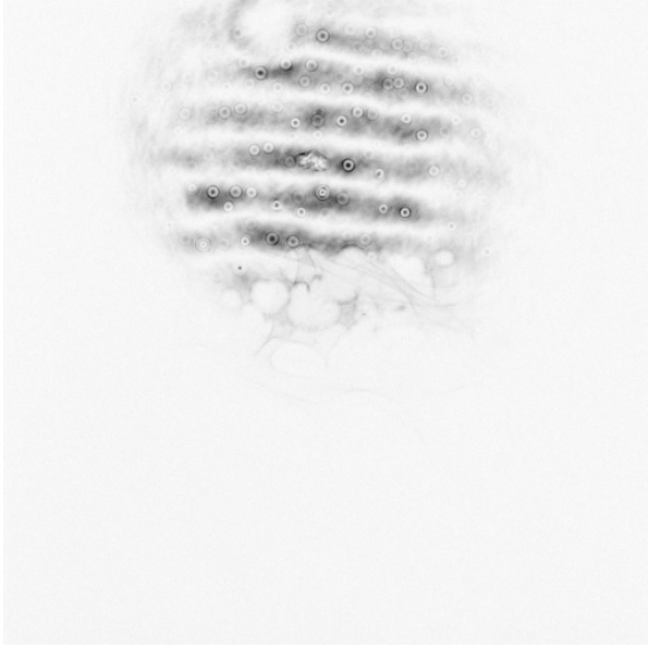
Attenuation: 1.41 * 10^{-7} , Acquisition time: 1s, gain: 0x, Polarizer D = 45^\circ Comment: Fringes clearly visible
