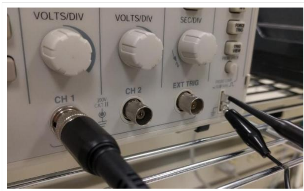
figure 3. Oscilloscope probe comp setup
