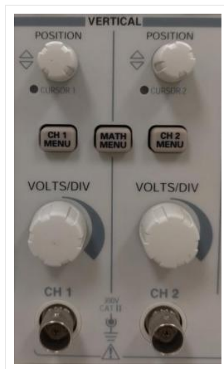
figure 5. Vertical section controls
