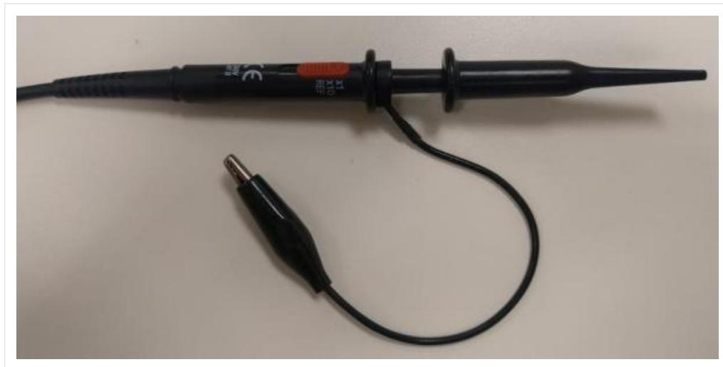
figure 2. Typical oscilloscope voltage probe
