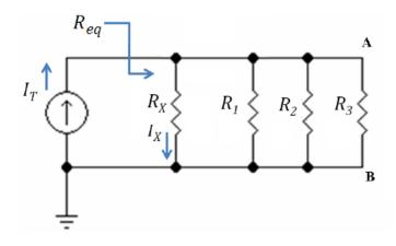
$$R_{eq} = \frac{1}{\frac{1}{R_X} + \frac{1}{R_1} + \frac{1}{R_2} + \frac{1}{R_3}}$$
