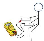
Measuring your body's resistance using an Ohmmeter connected to foil pads
