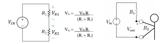
One application of voltage dividers is in circuits that sense the physical world. Replace  $R_2$  with a resistor that varies based on some environmental parameter, such as temperature or ambient lighting, and you will be able to infer the quantity of interest just by measuring  $V_{out}$ .
