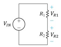
3. Complete Table 2 in your datasheet by calculating the expected value of  $V_{R1}$  and  $V_{R2}$  using the voltage divider formula, and then measuring these values with the DMM. Then compute the percent error using the formula provided.
