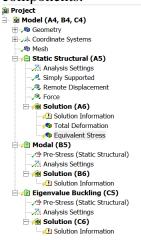
Now click on Solution under the Modal analysis and insert Total Deformation. Solve the model and you should see;
