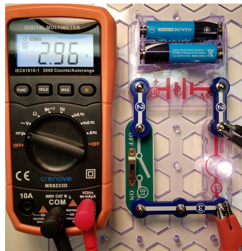
Figure 4a: voltmeter measurement with S1 closed
