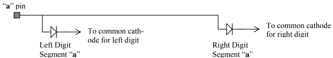
Figure Disp-iv: Display segment multiplexing.
