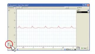
The Auto Scale button on the Tool bar (17) will automatically adjust the Y-axis scaling on ALL channels.
