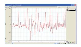
Small signal: Adjust the Range. If that doesn't work, readjust transducer strap or try placing the MLT1010 on your thumb.
