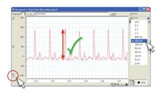
Scale the Y-axis (amplitude) if desired, using the Scaling buttons 21.
