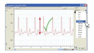
Scale the Y-axis (amplitude) if desired, using the Scaling buttons (21).
