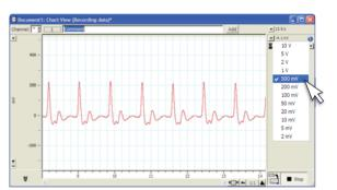
Verify the new range is appropriate for your signal. The maximum height should be 1/3 to 1/2 of the total range.
