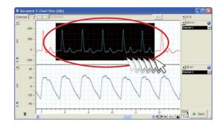
To select data in a second channel while retaining the first selection, drag the mouse over the second channel while holding down the Shift key on the keyboard.
