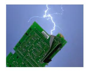
Moisture, temperature, materials and movement combine to create static charges which can damage printed circuit boards (PCB) and other sensitive equipment.
