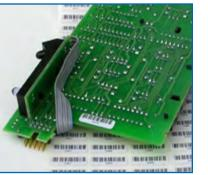
Printed Circuit Board Labels -Bar code or alphanumeric identification of printed circuit boards are used for tracking production lots, warranty information, product authentication, and registration applications.
