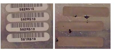
After Testing Results: New generation Polyimide Label (left) vs Standard Polyimide (right)
