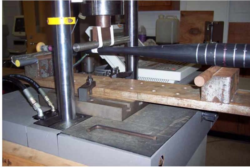
Figure 10 Three-point bend fixture
