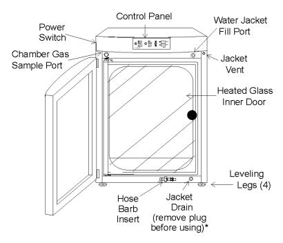
Figure 1-1 Water Jacket Incubator
