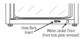
Figure 4-10, Water Jacket Drain and Hose Barb Insert
