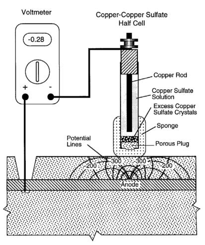
Figure A1. Apparatus for half-cell potential measurement, described in ASTM C 876.
