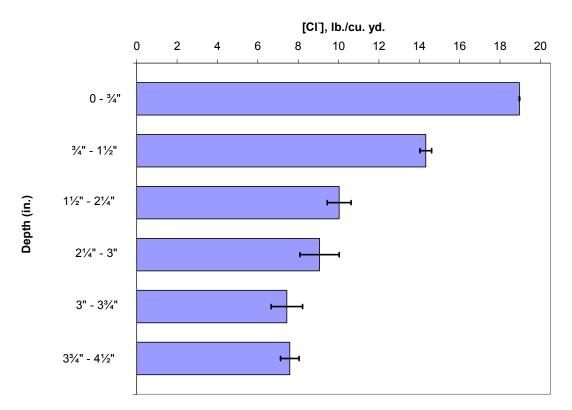
Figure 63. Chloride profile for SR 90 MP 61.304 (Price Creek).
