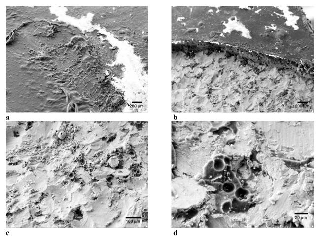
Figure 49. Green-epoxy-coated samples: (a) general view of the surface,  $100 \times$ ; (b) region where part of the epoxy coating was removed,  $100 \times$ ; (c) condition of the steel underneath the epoxy,  $302 \times$ ; (d) detail of corroded area and pits present under the coating,  $1330 \times$ .
