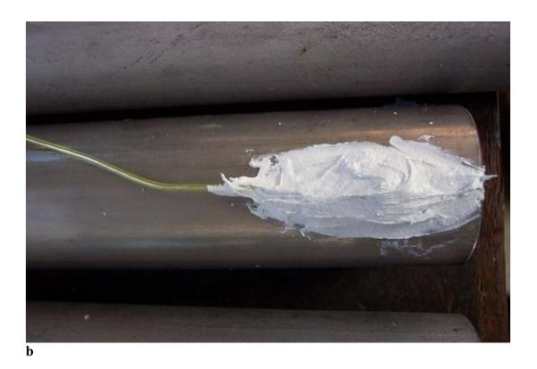
Figure 8. Electrical connections made to the stainless steel hollow specimens. Connections were made at the side of the dowel (a) and sealed with epoxy (b) before casting.
