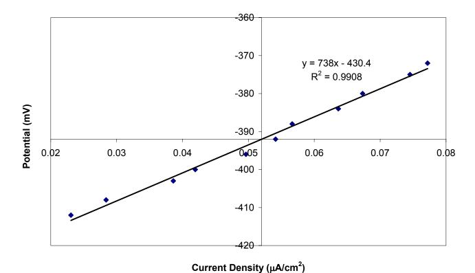
Figure 53. Linear Polarization Resistance, WSDOT slab, Specimen C.
