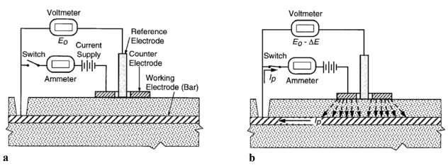
Figure A2. Three-electrode Linear Polarization Resistance method. (a) Measurement of the open-circuit potential (half-cell potential); (b) Current applied to the counter electrode to produce a small change in voltage  $\Delta E.(12)$
