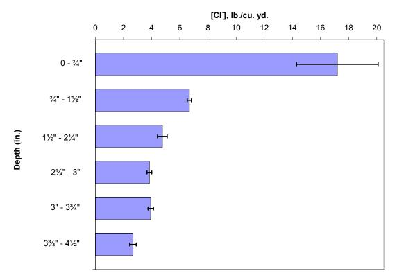
Figure 62. Chloride profile for SR 90 MP 91.324 (Elk Heights).
