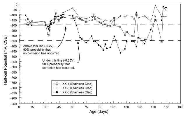
Figure 18. Half-cell potentials of stainless clad steel bars in Chloride ponding at 40-43°C.
