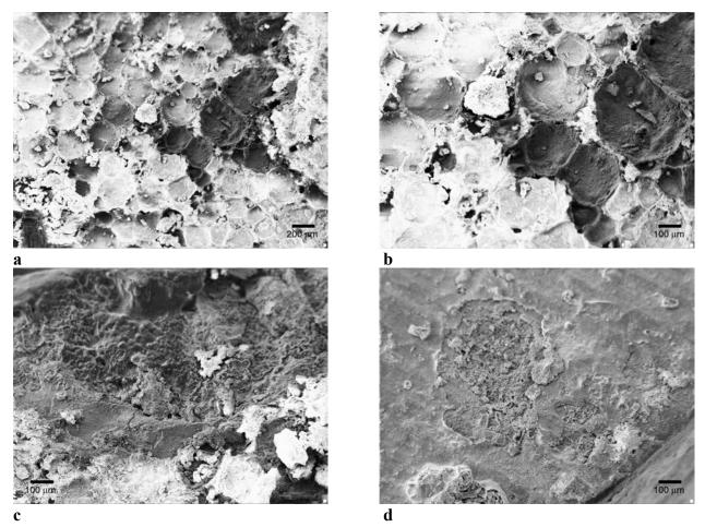
Figure 44. Carbon steel samples. (a) heavy corrosion along at the dowel surface, magnification =  $100\times$ ; (b) same region,  $200\times$ ; (c) different region at the surface,  $200\times$ ; (d) corrosion at the bar end,  $100\times$ .
