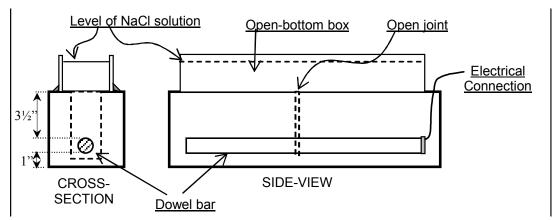
Figure 9. Experiment setup to accelerate corrosion using chloride ponding.
