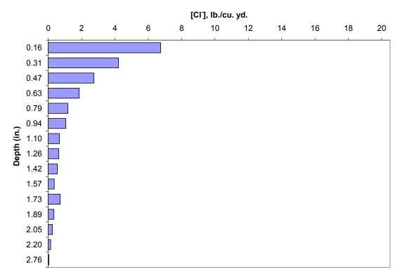
Figure 58. Chloride profile of the grout used for dowel bar retrofit (Core #3).
