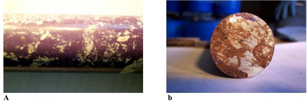
Figure 40. Epoxy-coated dowel (purple). (a) General view of the center region; (b) Corrosion was verified at the end region, underneath the epoxy seal.
