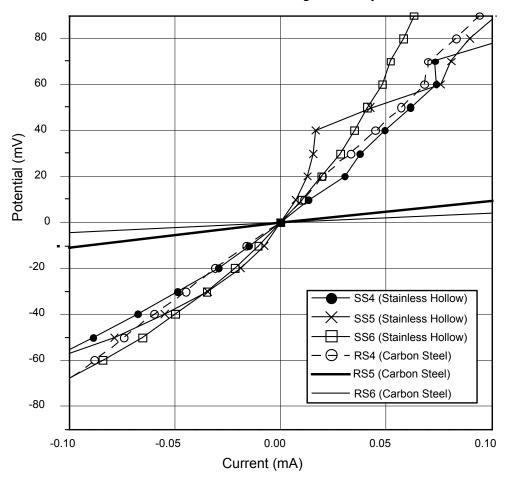
Figure 20. Linear Polarization of the carbon and stainless steels at 40-43°C.
