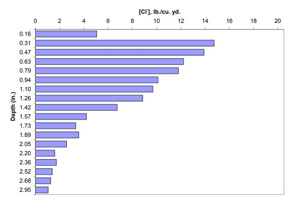
Figure 57. Chloride profile of the slab concrete (Core #2).
