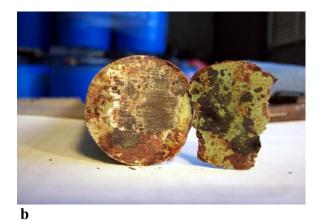
Figure 42. Epoxy-coated dowel (green). (a) General view of the center region; (b) Corroded edges and corrosion underneath coating at the end of dowels.
