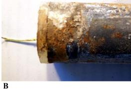
Figure 36. Carbon steel dowels. (a) Center region below joint (b) End with electrical connection.
